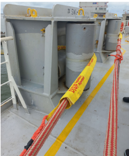
Figure 4: Chafe sleeve on the outer fore spring where it passes through the fairlead.
