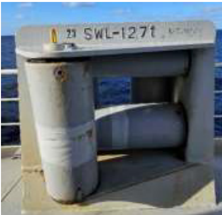
Figure 3: Five-roller universal fairlead on board YENISEI RIVER. This fairlead was involved in the accident.
