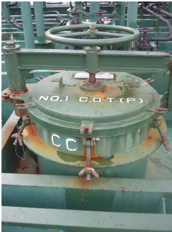
Figure 2: COT No. 1P access hatch and trunk.
