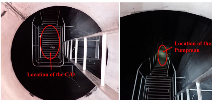
Figure 4: No. 6 S CT access ladder. The vertical ladder from the cargo tank dome to the upper platform is shown in the photograph on the left. The inclined ladder between the upper platform and the second platform is shown in the photograph on the right. The locations where the C/O and Pumpman were found are circled in red. The OS2 was found lying under the Pumpman.
