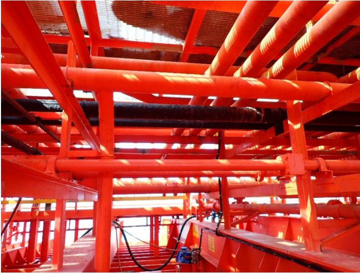
Figure 3: Grating and cargo pipelines above the cargo tank dome for No. 6 S CT.
