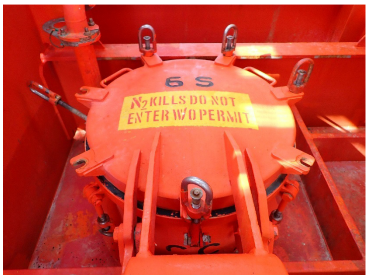
Figure 7: No. 6 S CT access hatch. Every cargo tank access hatch on board TRF KASHIMA was marked with "N2 KILLS" in addition to the warning required by the Company's enclosed space entry procedures.
