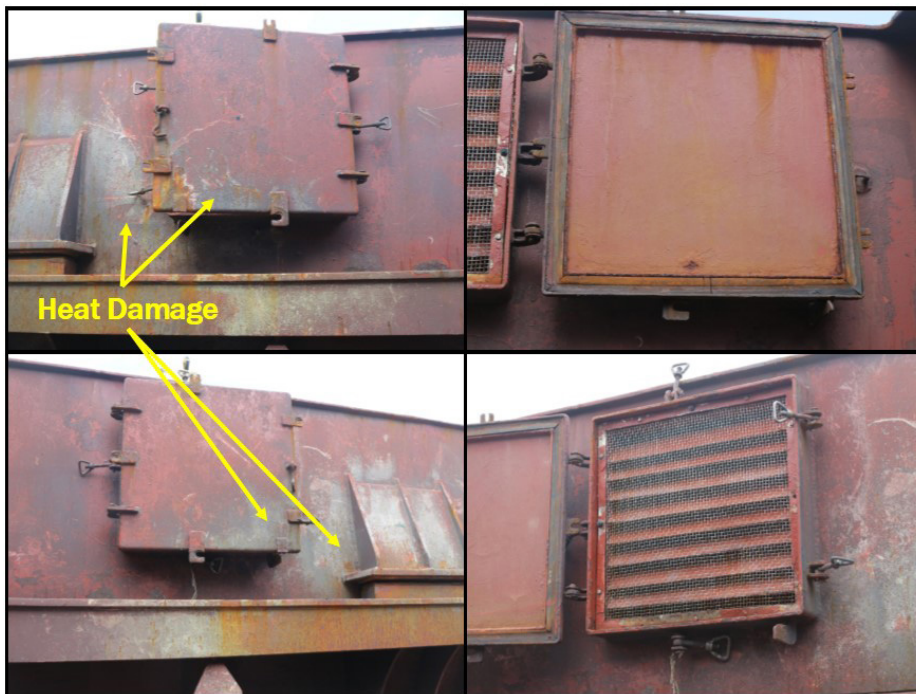
Figure 5: Port and starboard ventilation hatches for Cargo Hold No. 1. Heat damage present on exterior side of hatch only.
