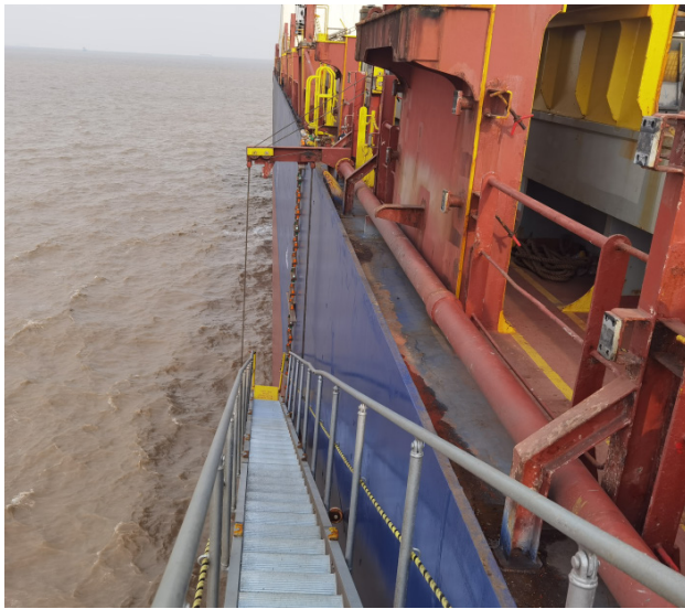
Figure 5: Starboard side accommodation ladder.
