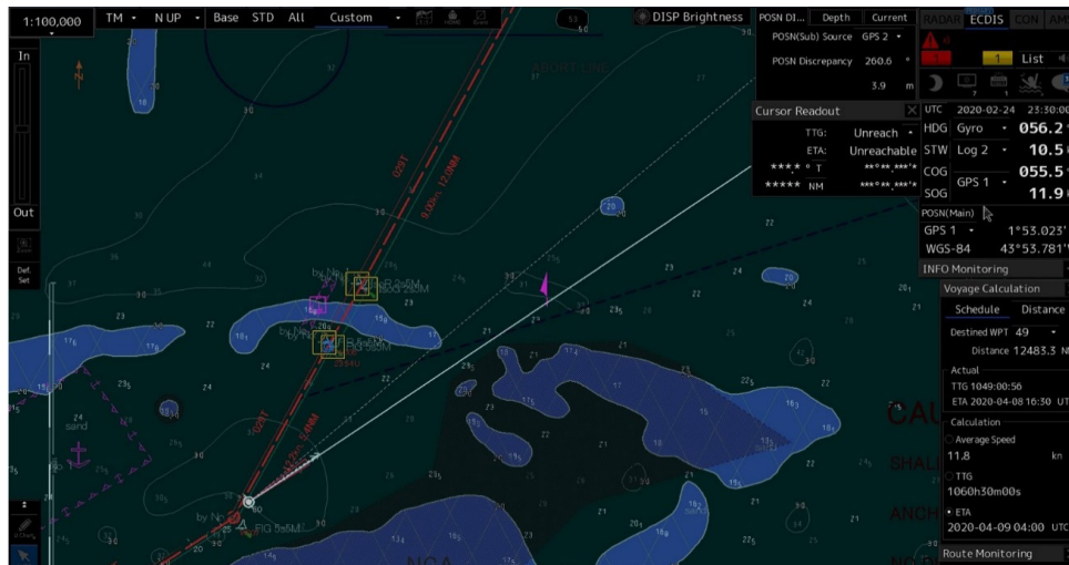
Figure 3: Position of STELLAR BANNER at 2030 when passing buoy No. 6 as shown on ENC BR321600. The charted depths in the gap between the two sandbanks are 21-23.5 m. The lighter colored areas are where the charted depths are 20 m or less. (Source: STELLAR BANNER VDR information.)
