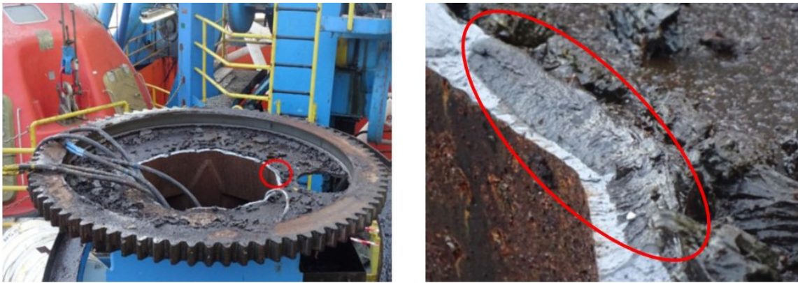
Figure 5: Top of the remaining section of the pedestal and a close-up of the area where the weld was found. The welded area is circled in red.
