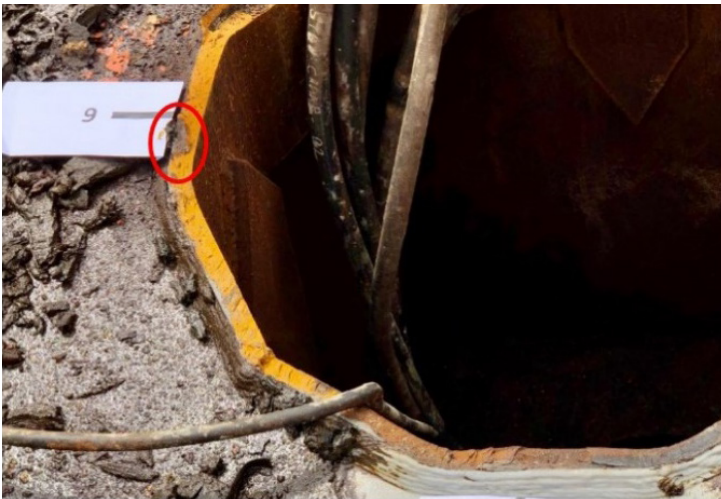
Figure 6: Top of the remaining section of the pedestal showing the area stained by grease (circled in red).
