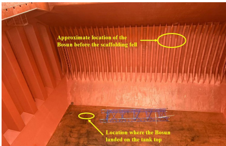
Figure 2: The approximate location of the Bosun before the scaffolding fell and location where the Bosun landed on the tank top inside of CH No. 3.
