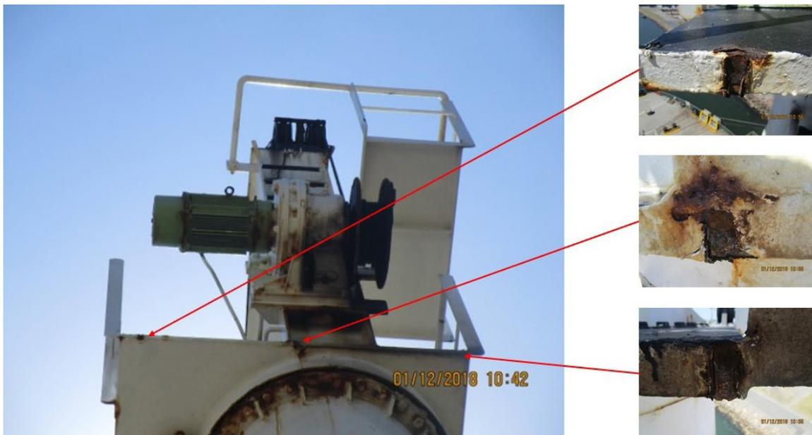
Figure 5: Portside provision crane showing the locations of the failed welds and the corrosion where the brackets were welded to the main platform. The Bridge Deck is to the left of the crane.
