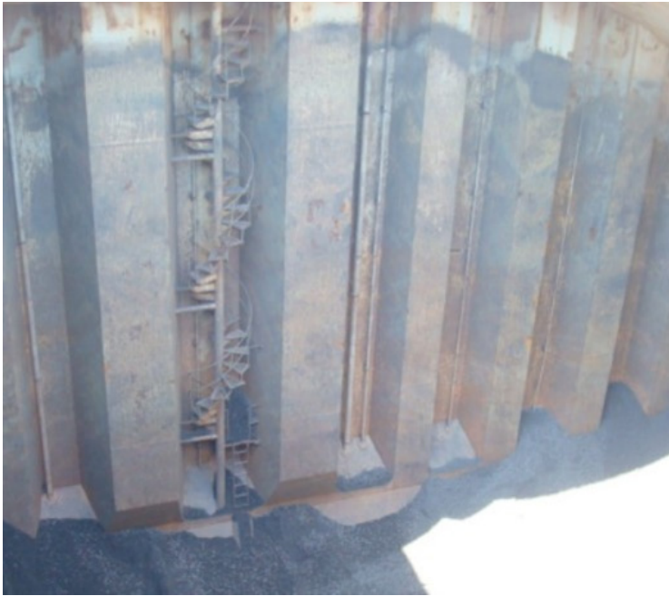
Figure 2: Australian ladder fitted in a cargo hold similar to Cargo Hold No. 5 aboard OURANIA LUCK. At the time of the incident, the hold was empty.
