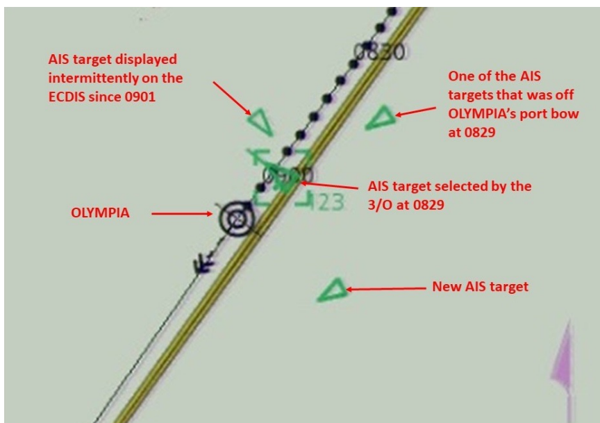
Figure 4: Portion of OLYMPIA's ECDIS display at 0915 immediately before the ship started turning to starboard. The AIS target off the ship's port beam had not previously been displayed.
