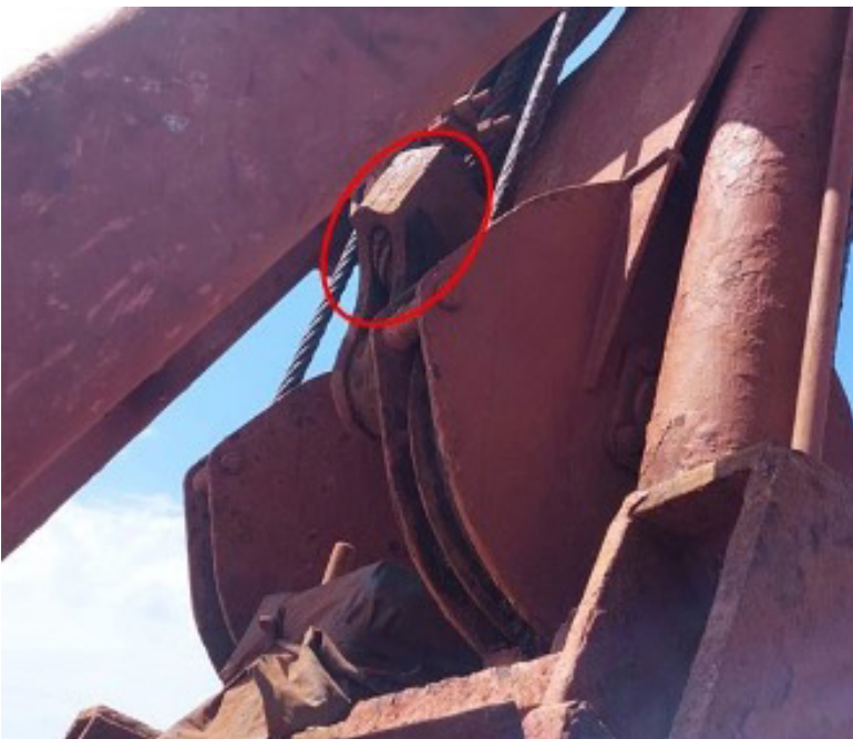
Figure 5: Dead end of the grab wire inside the wedge socket (circled in red).
