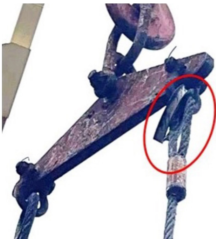
Figure 4: Dislodged thimble on grab wire for grab No. 1.
