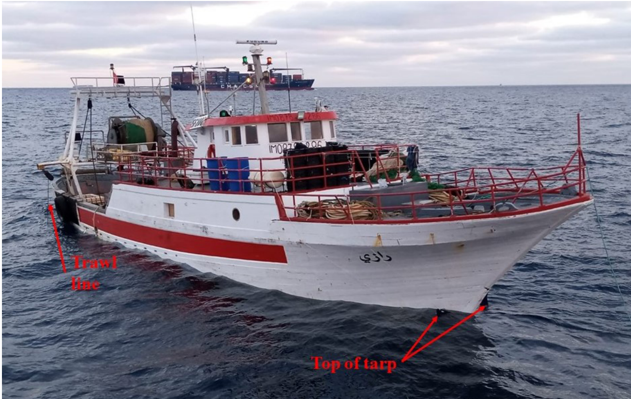
Figure 4: The location of the tarp over the lower portion of the stem and one of the two trawl lines. Note: In addition to the green light over the white light on the mast, there is also a red over a red light being displayed. The ship in the background is not MANTA HULYA. (Source: Tunisia Coast Guard)
