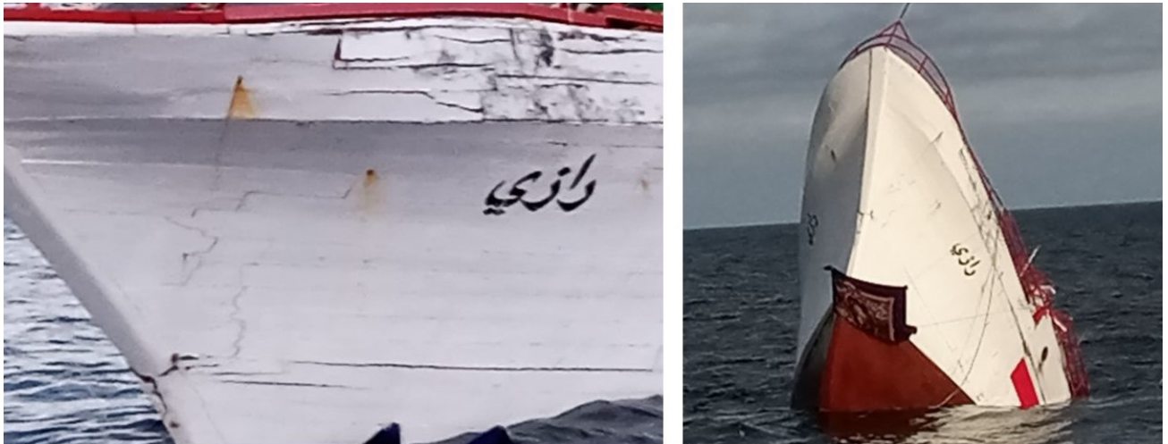
Figure 6: RAZI's hull, port side forward showing the damage to the stem and planking. The tarp that RAZI's crewmembers placed over the stem at the vessel's waterline is visible in the photograph on the right. (Source: Tunisia Coast Guard)
