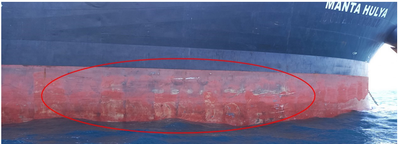
Figure 5: MANTA HULYA's hull, starboard side forward. The area where the scratches were observed are circled in red. (Source: Tunisia Coast Guard)
