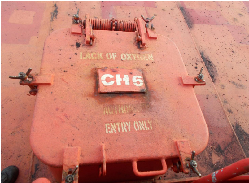
Figure 3: Access hatch for Cargo Hold No. 6.
