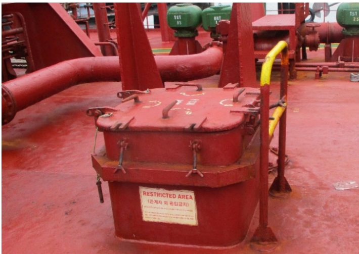
Figure 2: Access hatch to the aft ladder for Cargo Hold No. 1.
