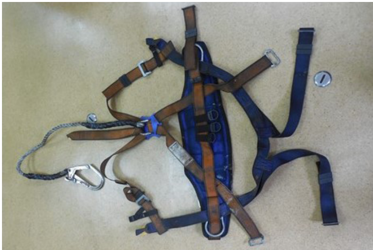
Figure 4: The safety harness worn by the Bosun when entering Cargo Hold No. 6 on 10 November 2020 (left) and the clip on the lifeline (right). The surface corrosion was in areas where the plating was missing.
