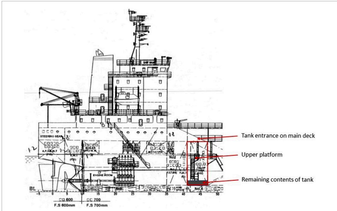
Figure 1: The slop tank is outlined in red.
