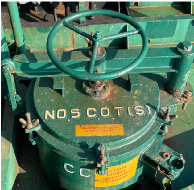
Figure 2: Tank access hatch cover (left) and Butterworth hatch cover (right) in closed condition.
