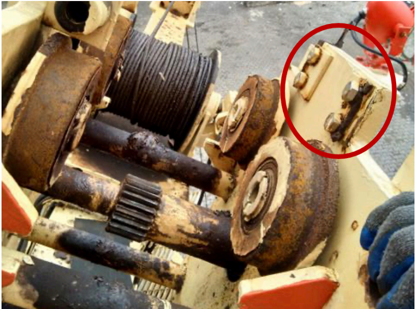
Figure 11: Photo of the travelling gear assembly. Note the missing aft stoppers circled in red.
