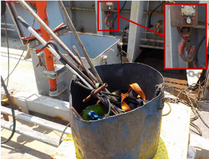
Figure 4: A photo of a bucket of tools aboard DERBY similar to what was being lifted by the Bosun. The mucking winch hook is highlighted in red.
