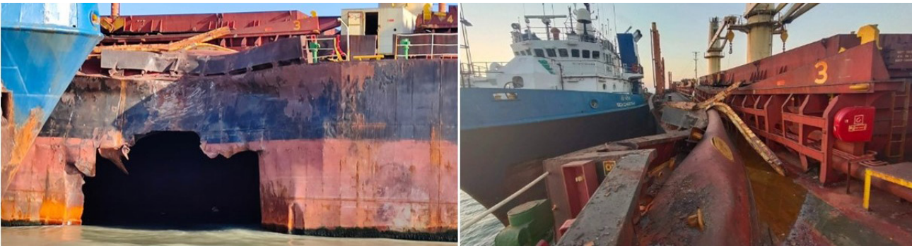
Figure 6: Damage to AVIATOR's port side shell and main deck.
