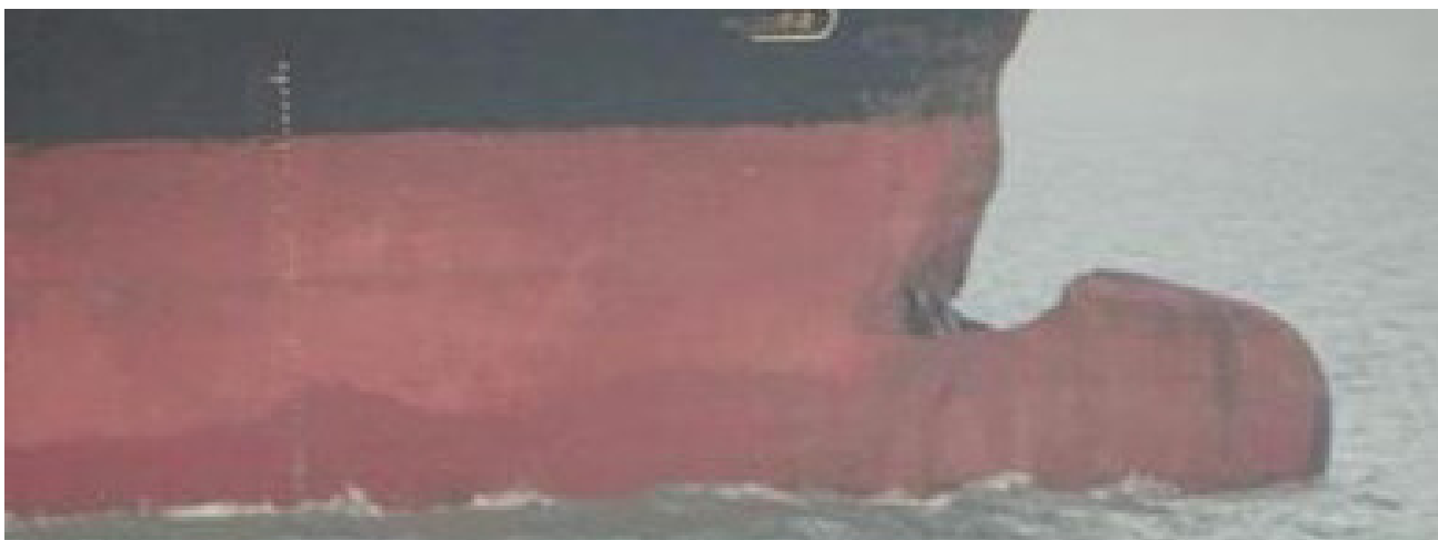
Figure 7: ATLANTIC GRACE's starboard side hull forward showing damage to the stem and bulbous bow. (Source: Indian Coast Guard)
