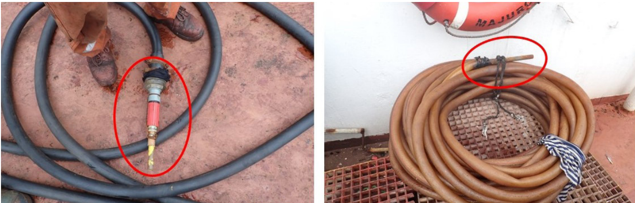
Figure 2: Hoses and nozzles that were used for cleaning the cargo holds.
