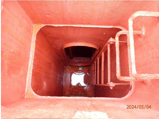
Figure 3: Vertical ladder and manhole leading to the catwalk at the top of Cargo Hold No. 4.
