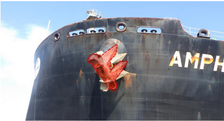
Figure 2: Photograph of AMPHITRITE's port anchor showing the position of the flukes when the anchor was stuck in the hawse pipe. The normal position of the flukes is indicated by the red image, which was added.
