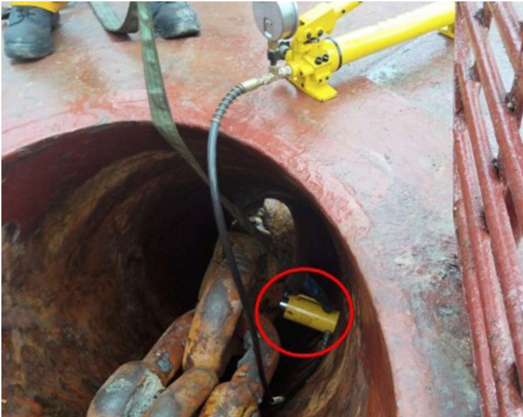
Figure 4: The port side hawse pipe showing the hydraulic jack (circled in red) in position on the forward side of the anchor shank. The hand pump for the hydraulic jack is on deck.
