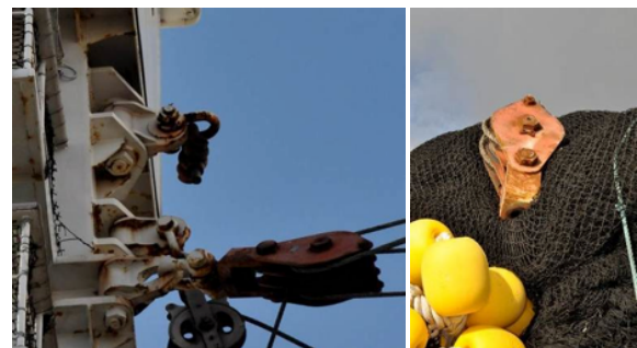
Figure 3: Upper topping lift, swivel pin remains attached to the joining shackle (left); fallen topping lift laying on fish net on the main deck (right).
