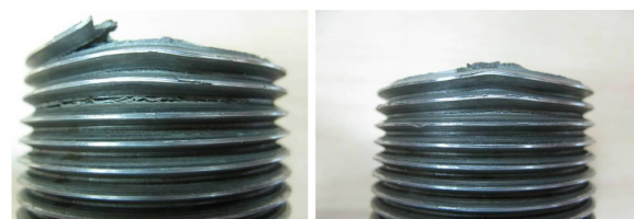
Figure 9: Threads on lower (left) and upper (right) pieces of the main boom topping lift (Source: UITL Report, page 6).
