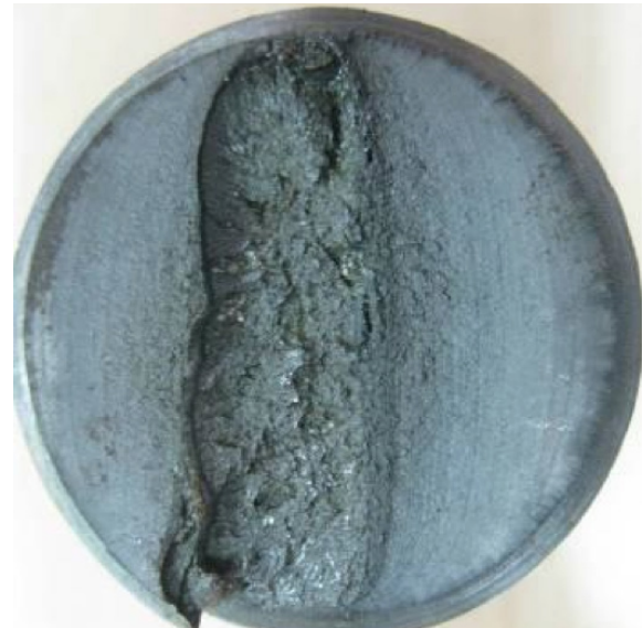
Figure 7: Cross section of main boom topping lift swivel pin showing final fracture zone in the center (Source: UITL Report, page 4).
